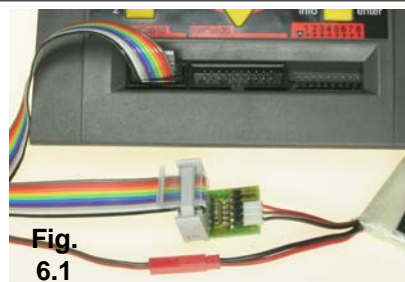
Fig. 6.1: Connection of 2s...4s-packs via a BalAd-TP4 or BalAd-Ko4 and a BalCab10-Verl to the nextGeneration, LiPoCard, LiPoProfiBal...
